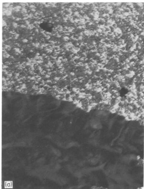
Figure 4 Dark-field micrographs of the region shown in Fig. 2 with the objective aperture on (a) spot A, and (b) spot B.
